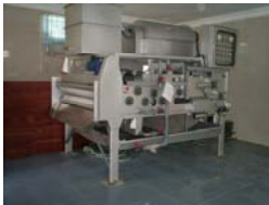
SLUDGE BELT PRESS
